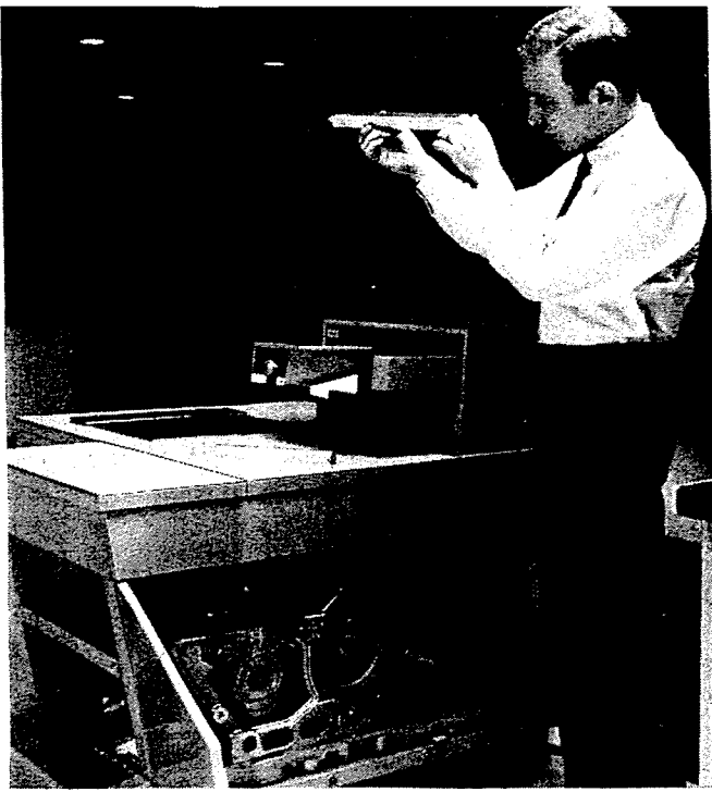
Looking for flaws in the corotron assembly used in a copier. This assembly gives the selenium drum a positive charge that prepares it to receive the electronic image.
