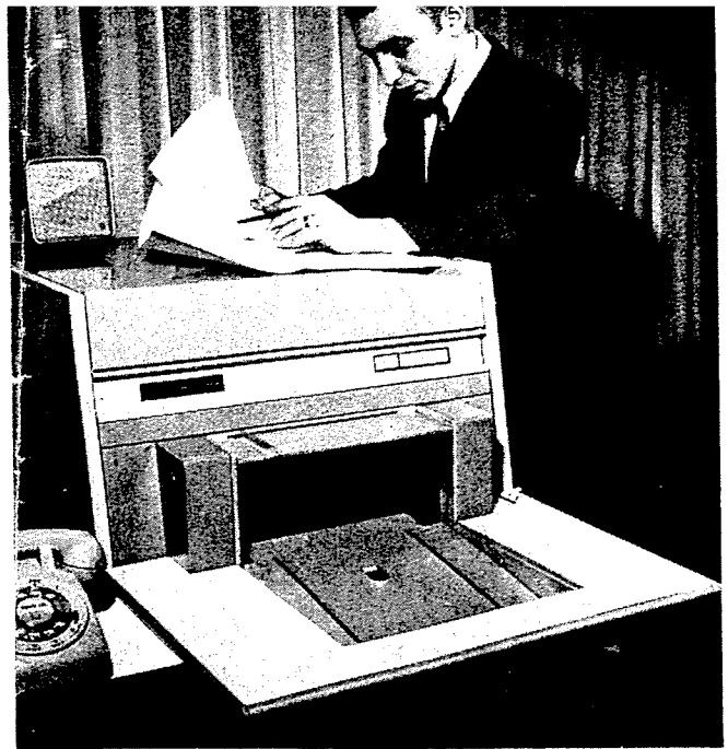
Preparing to tune up a long-distance xerography scanner, Levit traces a supervisory signal through the computer logic schematic.
